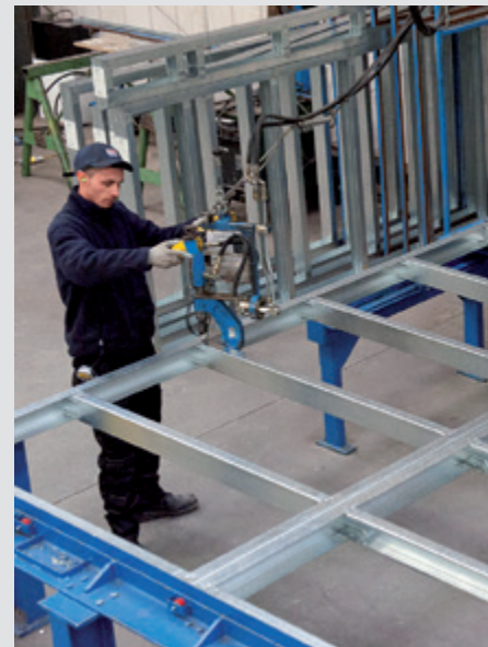
Manufacture of light steel wall panel within a factory environment after design freeze
